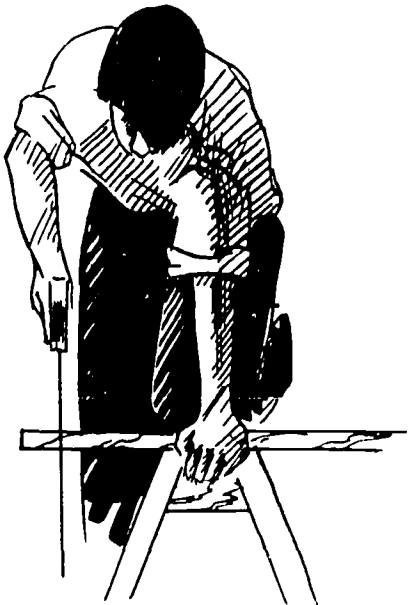
44.101 Figure 1-64.—Proper position for sawing a board to size.
